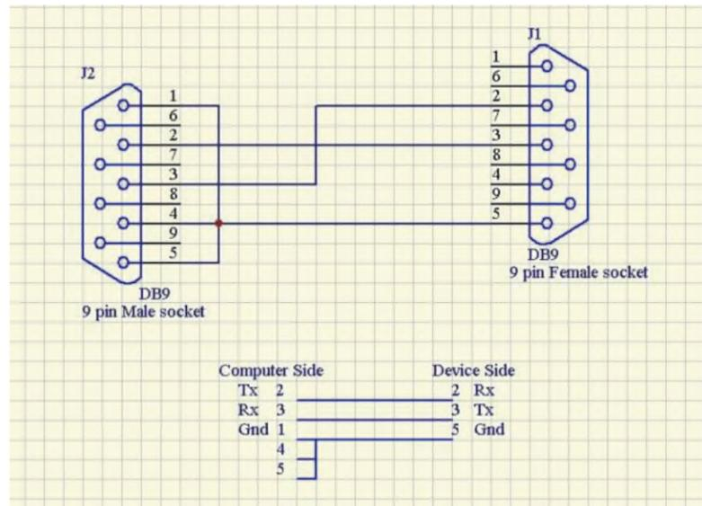
The operation mode of the maintenance port RS232 and the 485 port 2 on the rear panel of the relay is either-or mode. Once the connecting cable is plug into the terminal DB9 on the HYC2600-1 panel, the 485 port 2 stops working soon, and it starts to work again once remove the communication cable from the relay.
