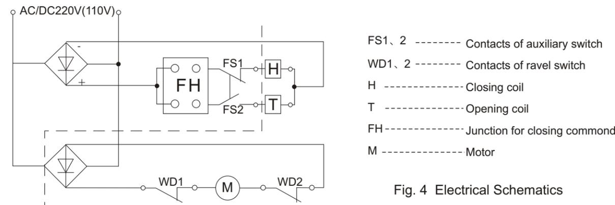
Fig. 4 Electrical Schematics
