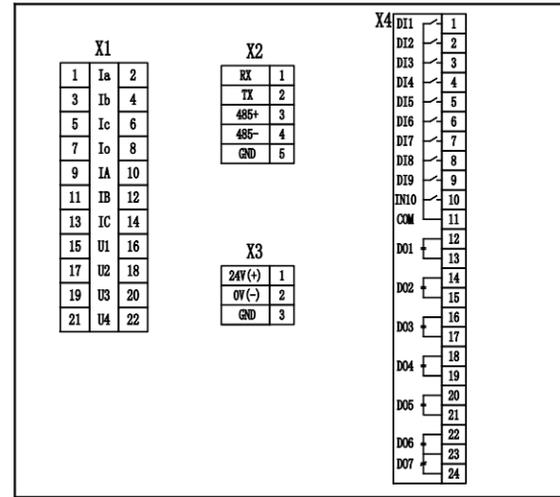
Fig.37 Rear Terminal Layout of Relay
