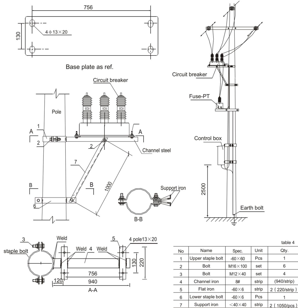
Fig.42 Single pole installation of ACR(CHZ-12) as ref.
