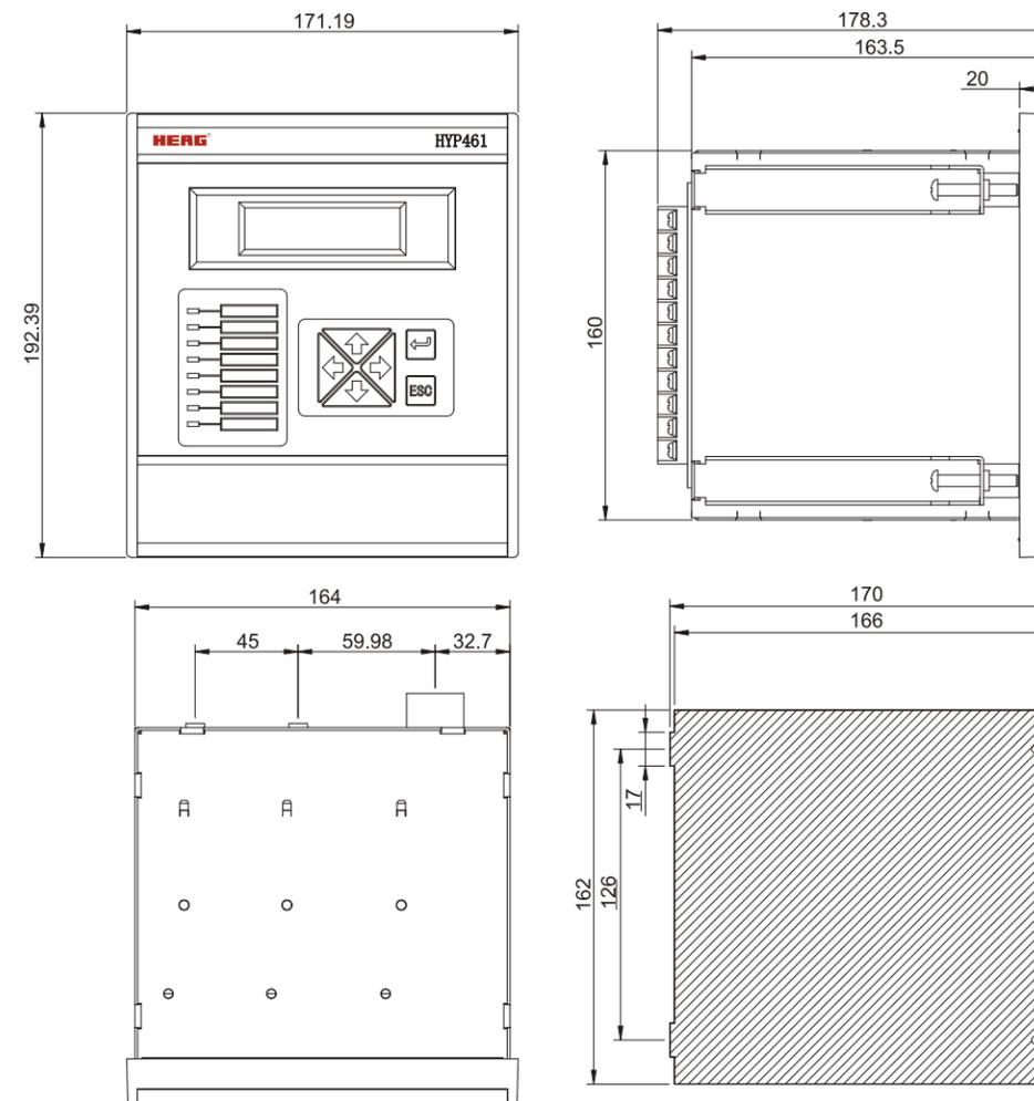
Fig.36. Outline & Installation Dimension of ACR Relay(unit: mm)
