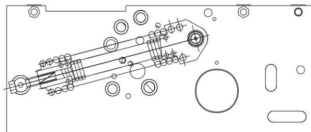
Fig.10-b Energy storage state of closing spring mechanism
