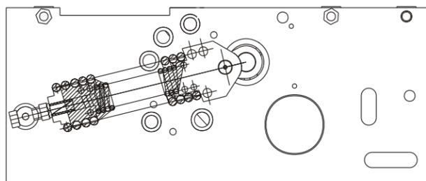
Fig. 10-a Energy non-storage state of closing spring
