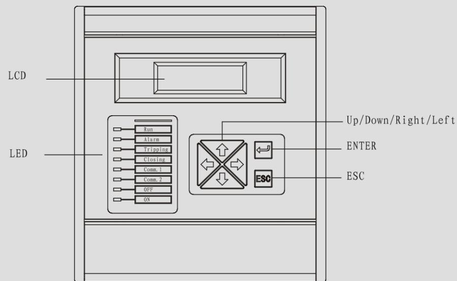
**Fig.1: ACR Relay Layout Drawing**
