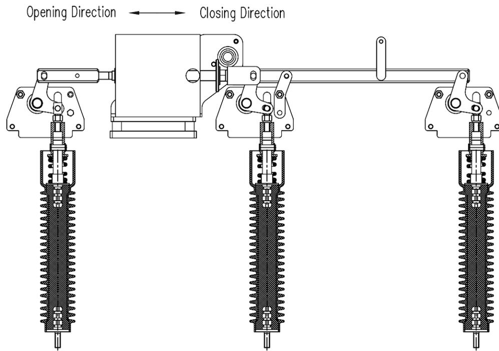
Fig.12 Internal driving system scheme
