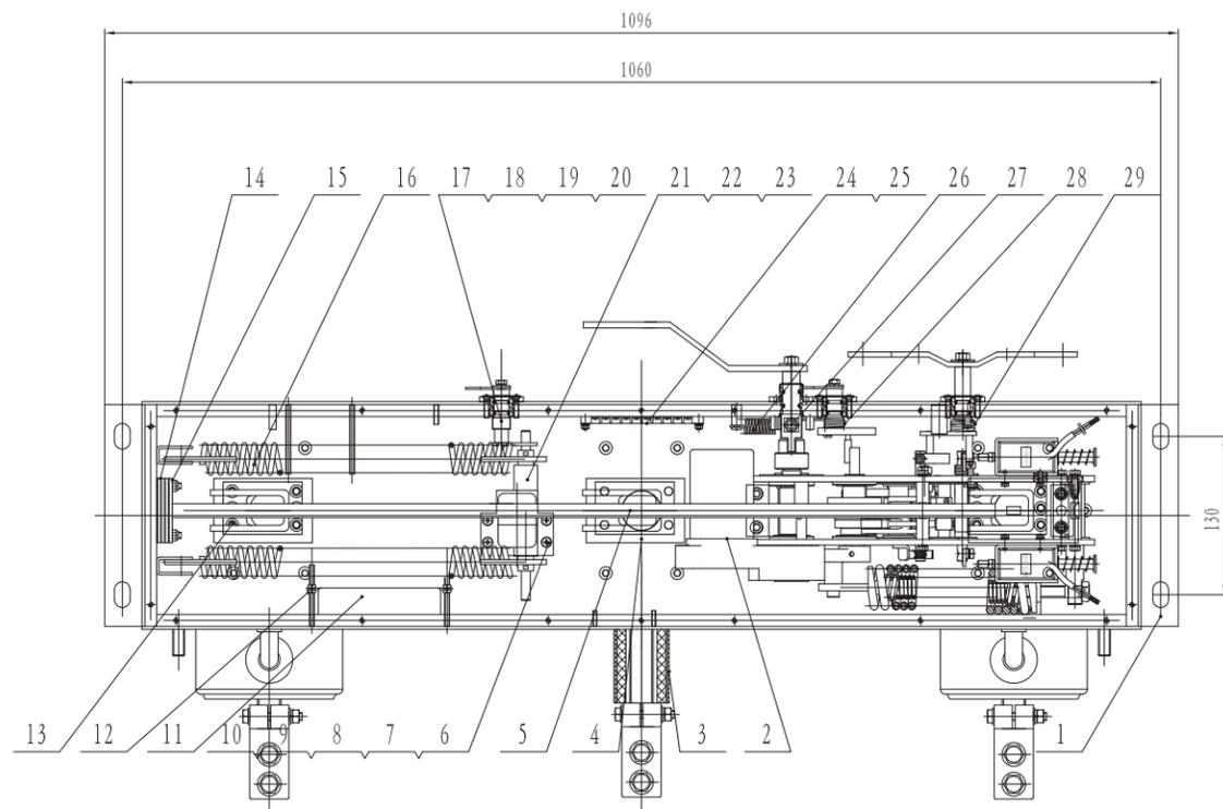
Fig.7 Spring Mechanism Structure for 24kV VCB of ACR(for example)
