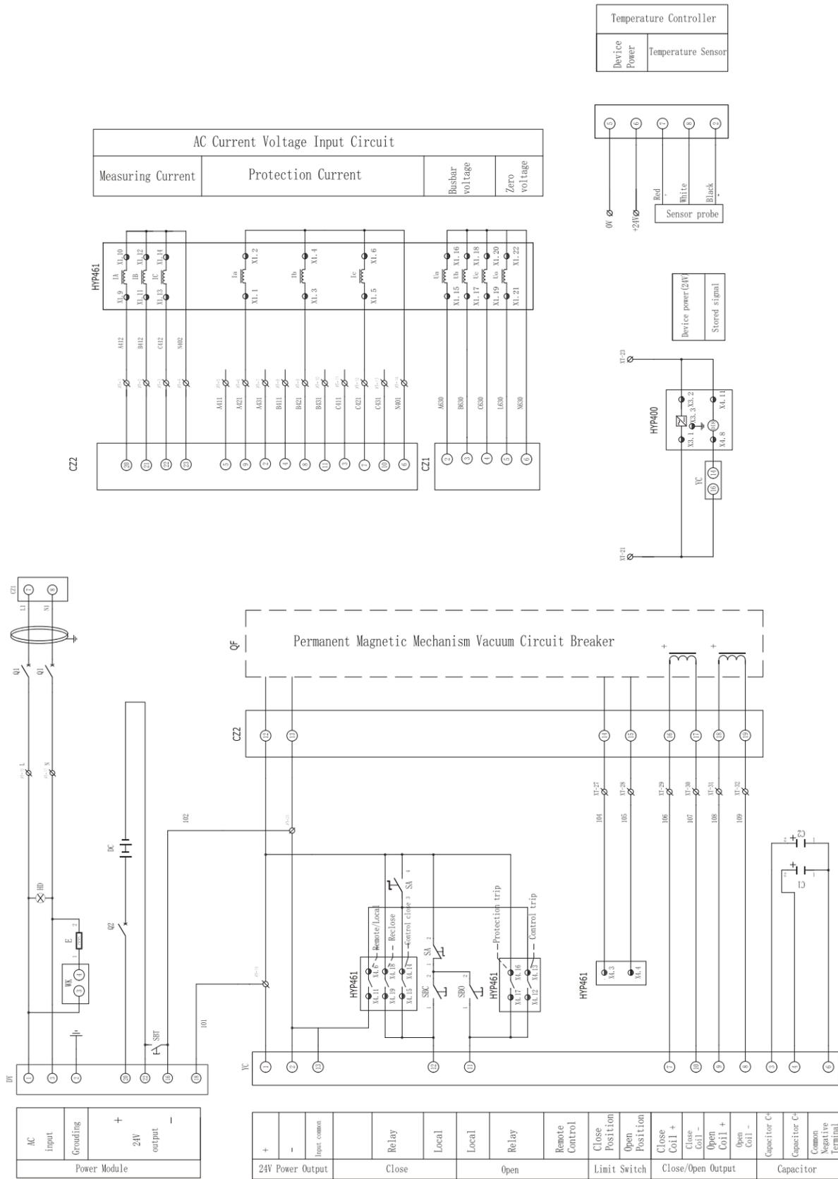
2-a) Principle control diagrams of ACR controller(Permanent Magnetic) as ref.
