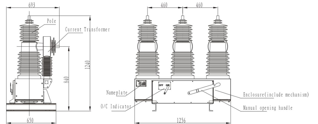
Fig.8-b Outline diagram of ZW37S-40.5 magnetic actuator VCB for ACR
