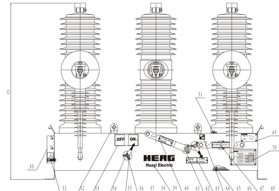
Fig.6, Outline Structure for 24kV VCB system(as example)
