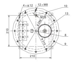
1.Conducting Rod 2.Standard Piece 3.Procelain Bushing 4.Cover 5.Procelain Bushing 6.Iron Core 7.Coil 8.Name Plate 9.Fixing sets 10.Stardard Oil Hole 11.PT Body 12.Conducting Rod 13.Mounting Base 14.Standard Piece 15.Sealing Cover
